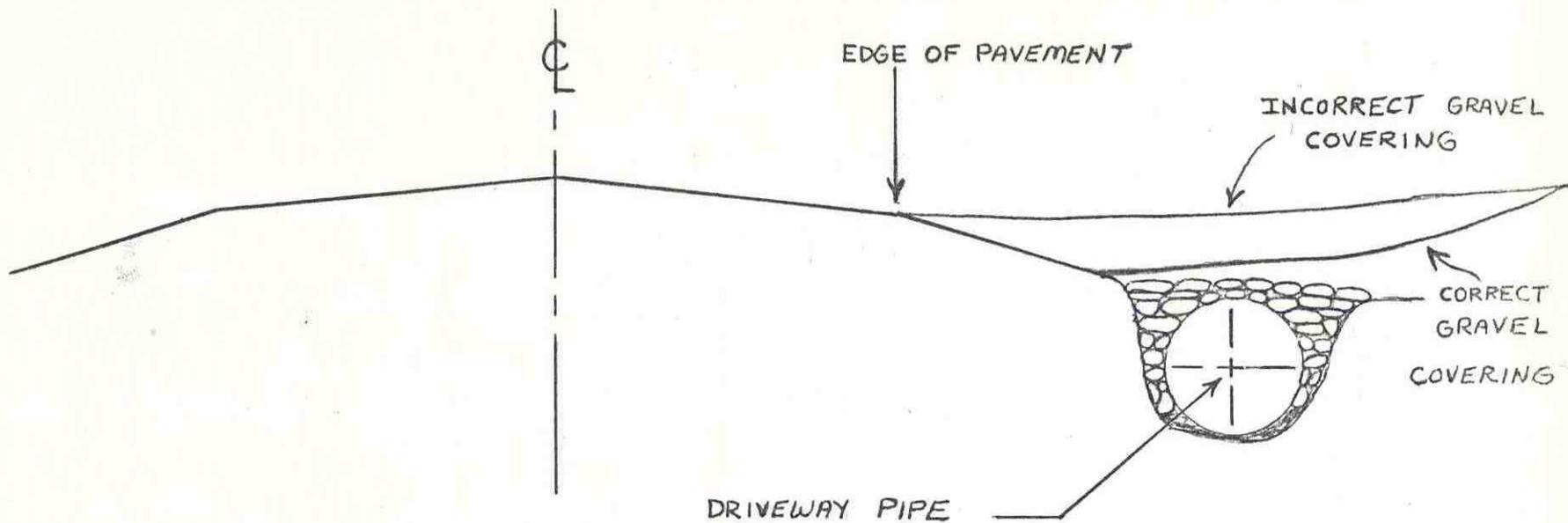
GRAVEL COVERING DRIVEWAY PIPE SHOULD BE FEATHERED TO MEET THE SHOULDER OF ROAD NOT THE EDGE OF PAVEMENT, THUS ALLOWING WATER RUN-OFF DOWN THE DRIVEWAY TO FLOW BACK TO THE DITCH, RATHER THAN OUT TO THE MAINLINE OF THE ROAD.
